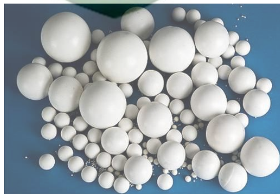
Gambar 2.7 Bola-bola penumbuk ( ball mill ) (Sumber : Chusnul azhari dkk, 2017)
