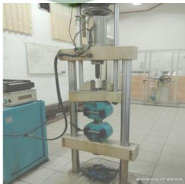
Gambar 3.9 Alat bending test
