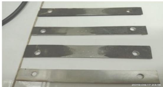
Gambar 3.11 Pelat strip stainless steel (AISI) 304
