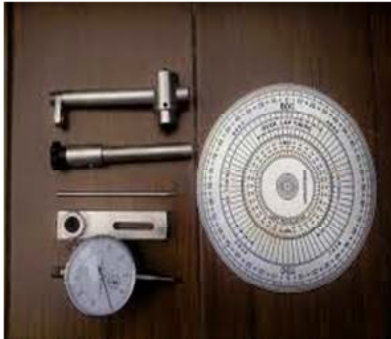
Gambar 2.21 Dial indicator, adaptor dial indikator, busur derajat
