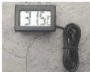
Gambar 3.6 Termometer Digital
