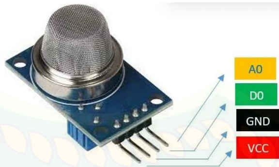
Gambar 2. 2 Pin Out MQ2
