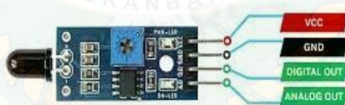
Gambar 2. 4 Pin Out Sensor Api
