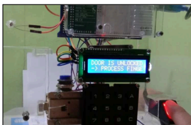
Fig. 7. The authentication process in the prototype
