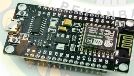
Gambar 2.1 NodeMCU ESP32
