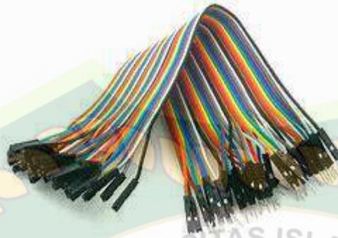
**Gambar 2.6** Kabel jumper *Male to Female*
