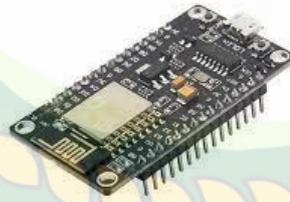
**Gambar 2. 1** NodeMCU
