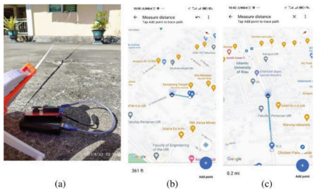
Fig. 7 Evaluation of sensor node (nRF24L01 radio frequency coverage)
