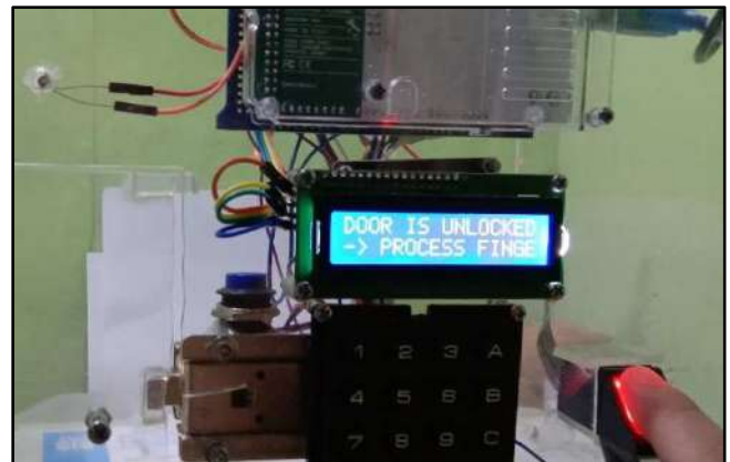
Fig. 7. The authentication process in the prototype
