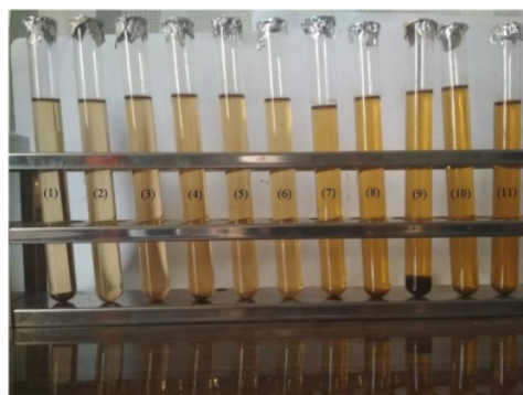
Figure 2. Hydrolysis results at a temperature of (1) 50°C (2) 60°C (3) 70°C (4) 80°C (5) 90°C (6) 100°C (7) 110°C (8) 120°C (9) 130°C (10) 140°C (11) 150°C
