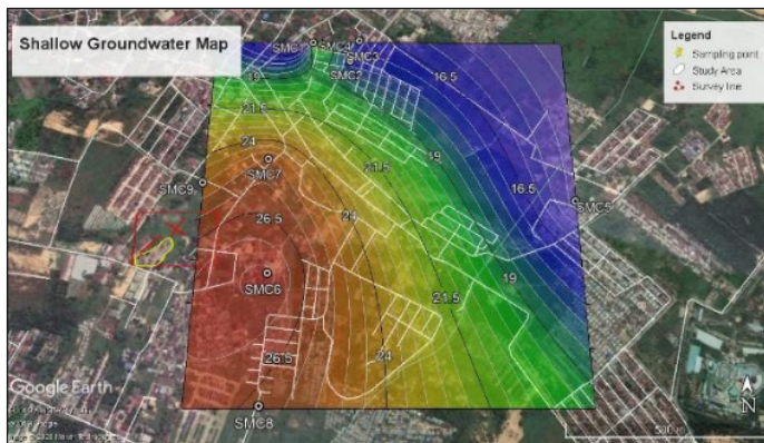
Figure 8. Groundwater elevation map that show the probability of contaminant migrate to Northeast from study area.
