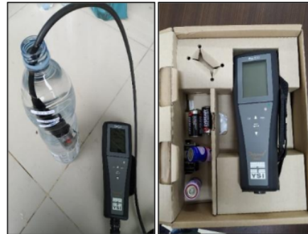
Fig 4. Equipment for groundwater quality analysis (Ph, temperature, TDS and conductivity).
