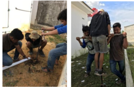
Figure 1. The sampling process using the hand auger method
