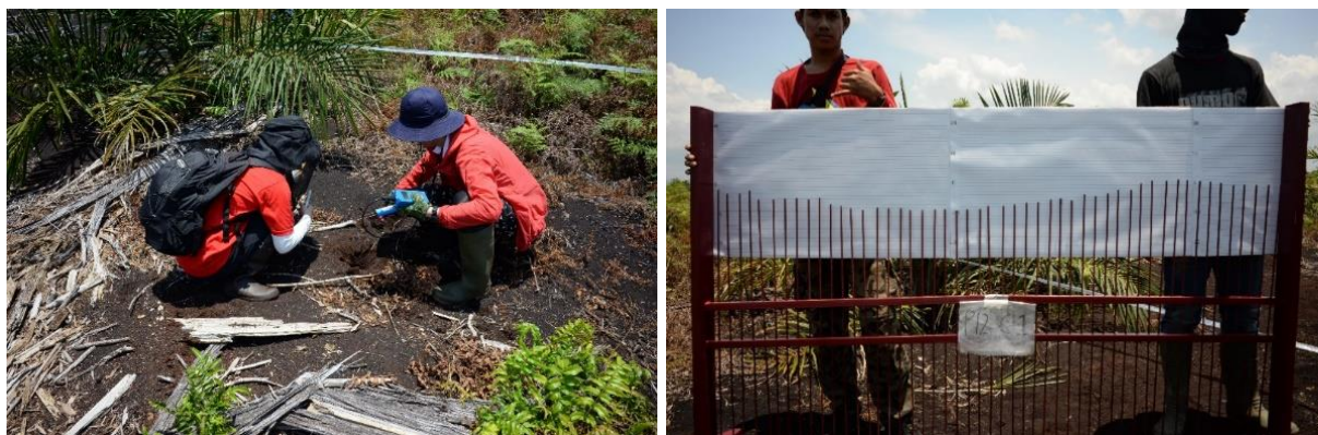
Figure 4. Measurement field. (left) Measurement of soil moisture with TDR, (right) Measurement of soil roughness with needle profiler.
