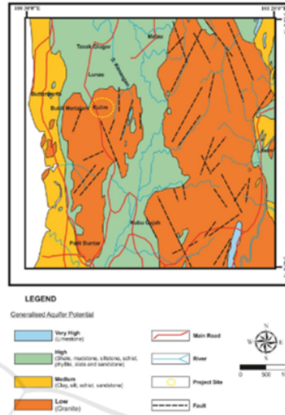
Figure 3: Geological Map of study area that consists of granite and surrounded by sedimentary rock and metamorphic rock (Hutchison, 1989).
