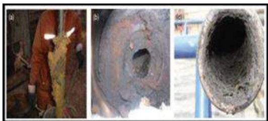
Figure 2: effect of wax deposits shown above (a) measuring drilling tubing, (b) intersection of the flow pipe, and (c) on the inside of the pipe.
