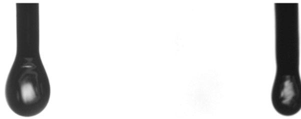
Figure 5—Oil drop shapes at 1000 and 1400 psi and 60 °C
