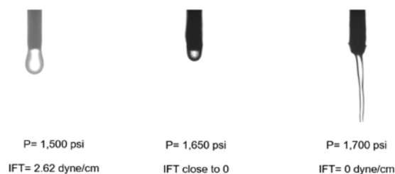
Figure 8. MMP by visual observation under IFT test at T = 60\text{ }^{\circ}\text{C} . 26
