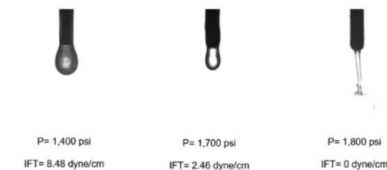
Figure 9. MMP by visual observation under IFT test at T = 66\text{ }^{\circ}\text{C} . 26
