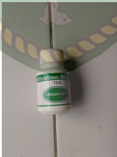
Gambar 3.9 Cairan calibrasi tds meter
